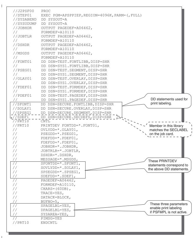
Figure 16. Sample PSF Startup Procedure with Security-Related Parameters Highlighted. A sample startup procedure is provided in SYS1.PROCLIB.
