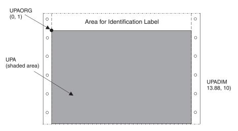
Figure 9. Page Layout for a Continuous Form
