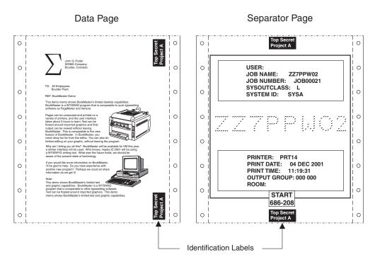
Figure 1. Print Labeling. Identification labels can be placed on the top, bottom, or sides of all pages within a job. This example shows a page from two different jobs.
